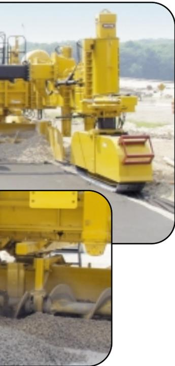
PS-4000 conveyor is designed to extend in seven seconds and the conveyor deflector directs the material for the paving operation.
