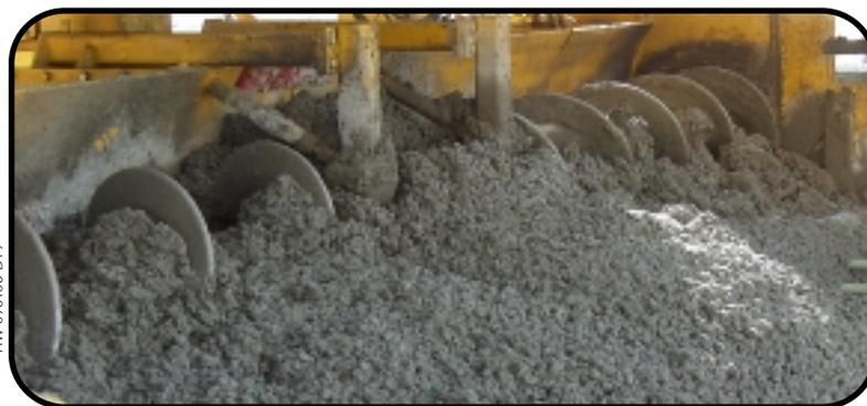
The spreading of either concrete or base material is quick and accurate with the reversible 20 in. (508 mm) diameter hydraulically powered split auger. The hydraulically pressure-compensated sideplates provide edge control and a spreading depth up to 19 in. (483 mm).
