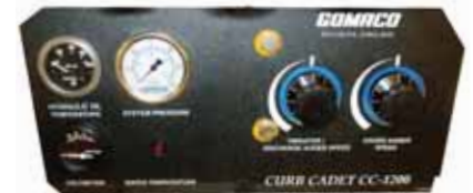
The vibrator adjustments and cross-auger knob are located on the front of the machine.
